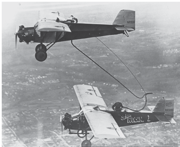
Airplane “St. Louis Robin 1” refueling in midair during an endurance test lasting from 13 July to 30 July 1929. The Robin set an endurance record with 420 hours, 21 minutes, and 30 seconds of continuous flight. Photograph, 1929. Missouri Historical Society Photographs and Prints Collections. Aviation 351. NS 30209. Scan © 2007, Missouri Historical Society.
